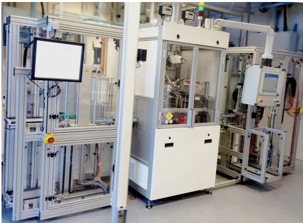
Fig. 6: Fully automated 1000 W/h ADE texturing pilot line machine produced by Nines-PV [16].
